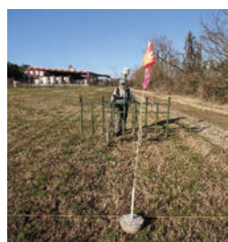
Figure 2. Jarrod running the magnetometer. Markers are used as a sight target so he can walk a straight line, which is important for proper data collection.
